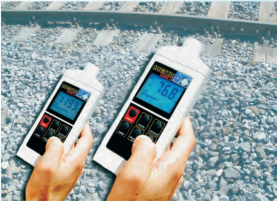
Evidently effective against squeaking and screeching: measurement prior to lubrication (left) and after application of Sintono® Terra HLK (right) .
