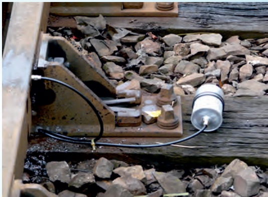
MicroMax® 120 installed at check rail
